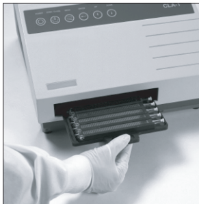
Load cassette tray into CLA-1 Luminometer
