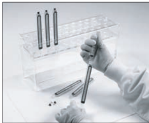
Draw photoreagent into Pettes
